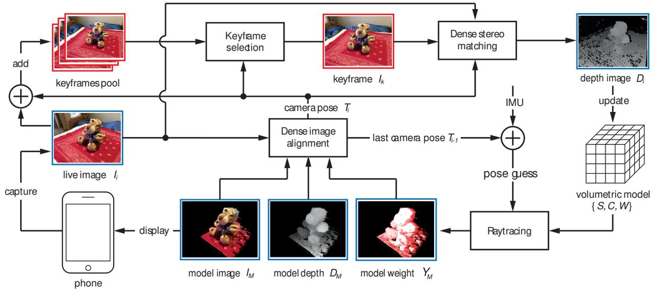
Fig. 2. System pipeline. See text for details.
