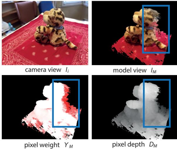
Fig. 4. Detail of the weighted image alignment scheme for camera tracking. Model view  $\{I_M, D_M\}$  is used for per-pixel alignment of camera image  $I_i$ . We downweight pixels corresponding to noisy parts of the model using the projection  $Y_M$  of weights  $W(p)$  stored in the TSDF.
