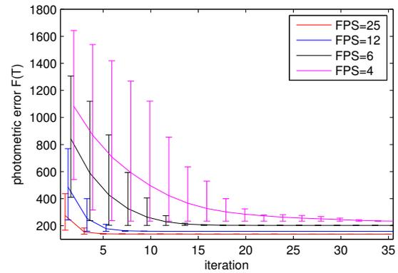
Fig. 6. Iterative alignment of live image during camera tracking. Our plots show the importance of maintaining high frame-rate camera tracking to ensure fast and precise convergence.
